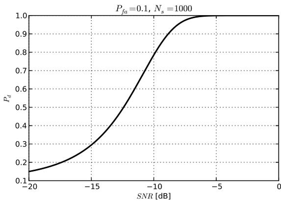
Fig. 3. Theoretical probability of detection  $P_d$  versus signal-to-noise ratio  $SNR$  for energy detector. Methods with better performance lie above the energy detector curve.
