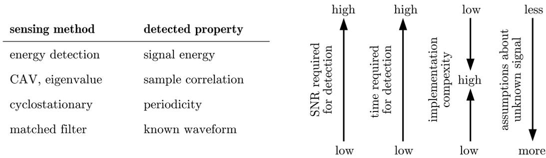
Fig. 1. Overview of spectrum sensing methods and their basic properties.
