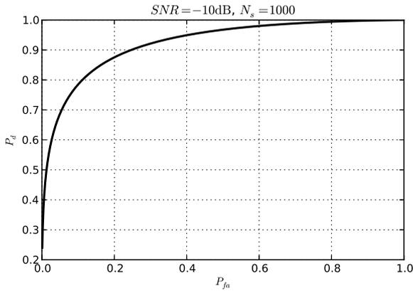
Fig. 2. Theoretical probability of detection  $P_d$  versus probability of false alarm  $P_{fa}$  for energy detector. This graph is also called *receiver operating curve*. Methods with better performance lie above the energy detector curve.
