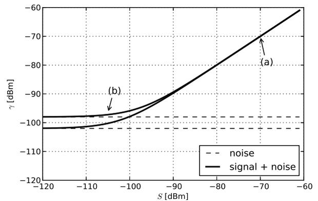
Fig. 5. Energy detector test statistic  $\gamma$  versus signal power  $S$  in log-log scale for two slightly different receiver noise floors. Detector output is relatively independent of noise power when the signal is strong (a), but with signal power at or below noise, reliable detection depends on accurate knowledge of the noise level (b).
