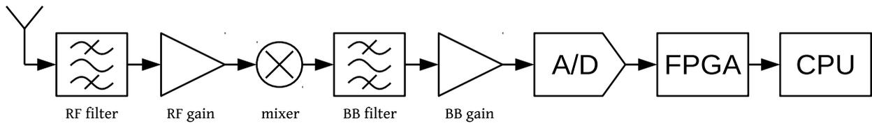
Fig. 8. A typical block diagram of a spectrum sensor based on a software-defined radio architecture. Analog front-end conditions the signal at radio (RF) and base-band (BB) frequencies. Digital part consists of a front-end implemented in a FPGA or an ASIC. High-level operations are done in software on a general-purpose CPU.
