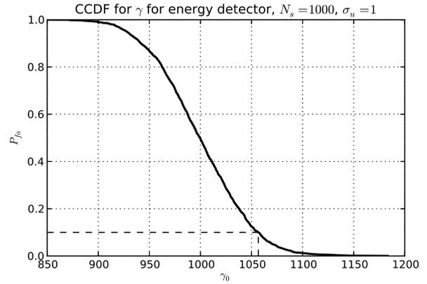
Fig. 4. Complementary cumulative distribution function for energy detector test statistic  $\gamma$  obtained through numerical simulation of 2000 measurements. Dashed lines indicate the threshold value  $\gamma_0$  for a chosen  $P_{fa} = 0.1$ .
