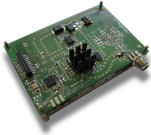
Fig. 7. SNE-ISMTV-UHF energy detector for the VHF/UHF band mounted on a VESNA sensor node is an example of a simple, low-cost analog implementation of a spectrum sensor.
