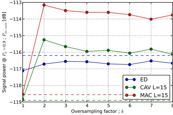
Fig. 6. Effect of oversampling on energy, CAV and MAC detectors. Dashed lines show  $P_{in-min}$  without impairments.
