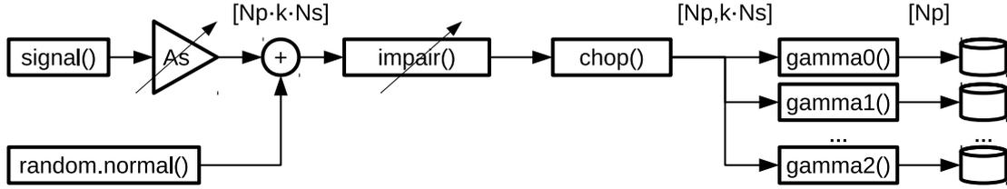
Fig. 1. Block diagram of the basic simulation process process ( $A_s$ ,  $\text{impair}$ ).
