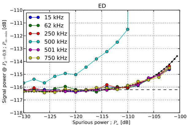
Fig. 3. Effect of spurious cosine noise component on energy detection. Small black dots shows the analytical result. Dashed black line shows  $P_{in-min}$  without impairments.
