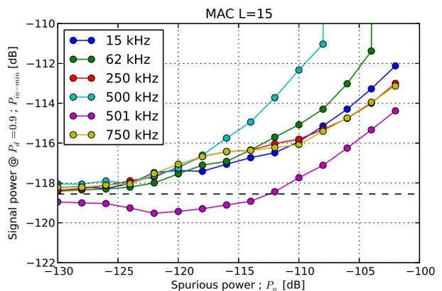
Fig. 5. Effect of spurious cosine noise component on the MAC detector. Dashed black line shows  $P_{in-min}$  without impairments.
