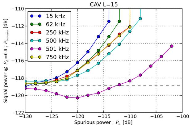
Fig. 4. Effect of spurious cosine noise component on the CAV detector. Dashed black line shows  $P_{in-min}$  without impairments.
