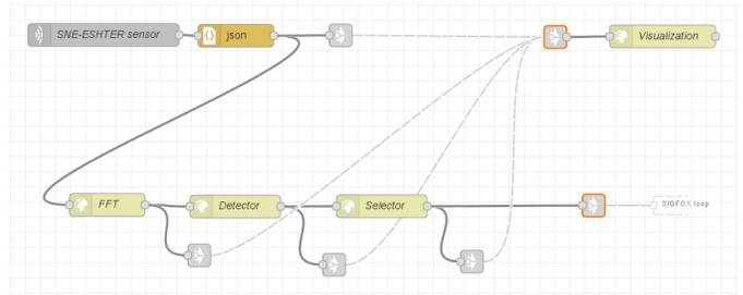
Fig. 3. Node-RED flow that receives spectrum data from a sensor, performs energy detection, calculates channel occupancy and performs visualization.
