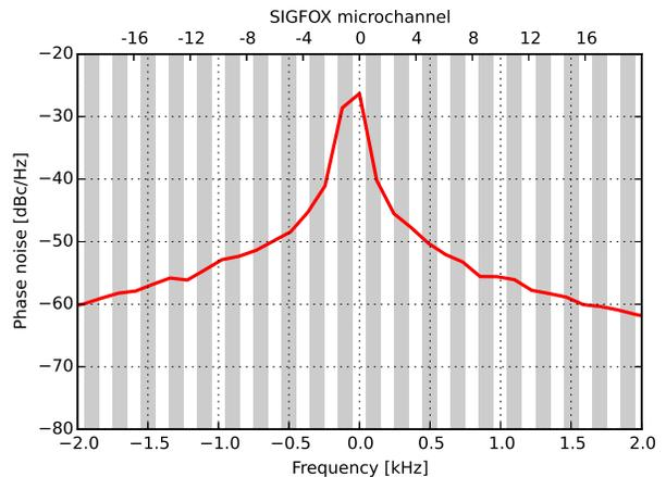
Fig. 7. Comparing phase noise of the spectrum sensor to the bandwidth of SIGFOX microchannels.
