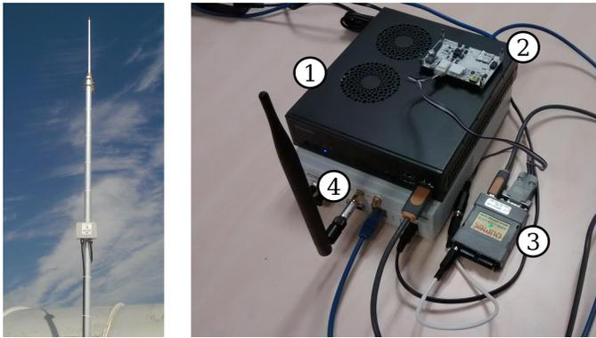
Fig. 2. Left: base station antenna. Right: SIGFOX test device - (1) miniature PC, (2) embedded board with modem firmware, (3) serial interface between PC and embedded board, (4) USRP N200 transceiver.
