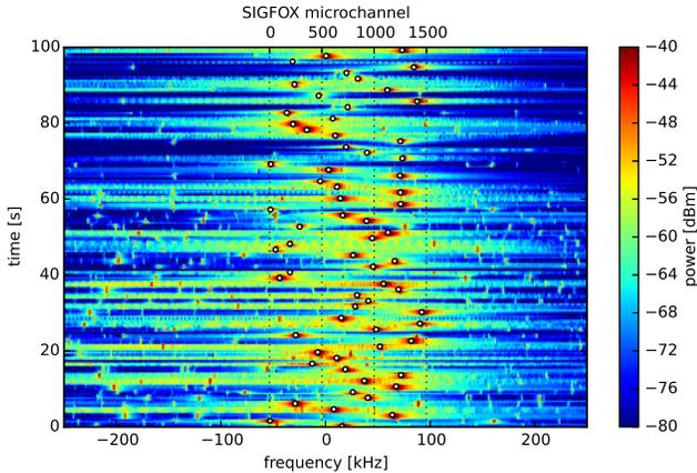
Fig. 5. Visualization of the spectrum sensing data from the sensor co-located with the transmitting device. Circular markers mark times and frequencies of SIGFOX frame transmissions (and associated packet context data).
