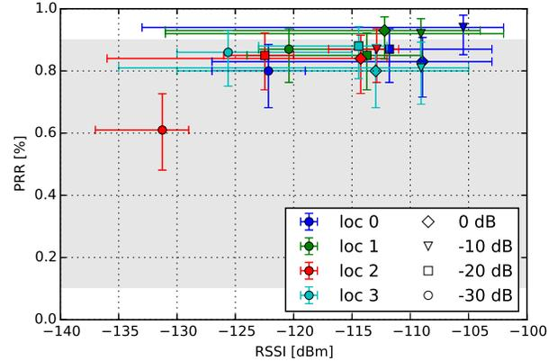
Fig. 6. PRR vs. RSSI for four locations and four transmit gains. Shaded region shows PRR range for intermediate links, with good links above and bad links below. Error bars show 99% confidence interval (N=100).
