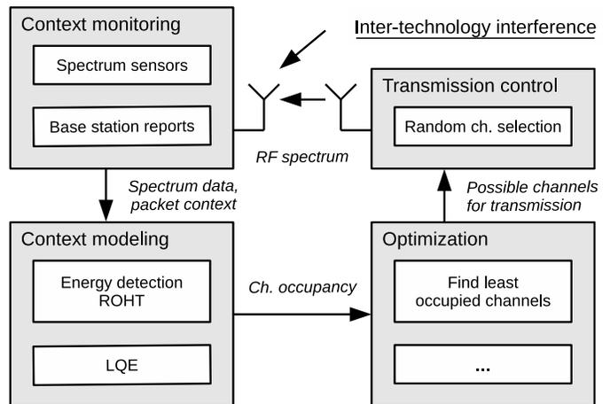
Fig. 1. Block diagram of the proposed architecture for optimization of UNB wireless communication with specific solutions adopted in our case study.
