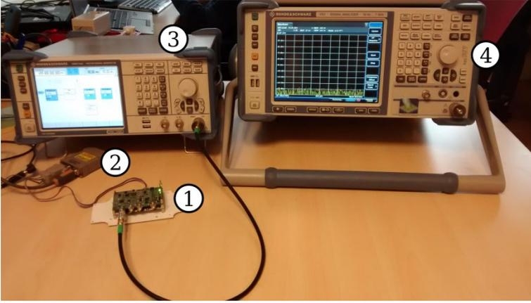
**Figure 2:** Experimental setup. (1) VESNA SNE-ESHTER sensor, (2) RS-232 interface, (3) vector signal generator, (4) signal analyser.
