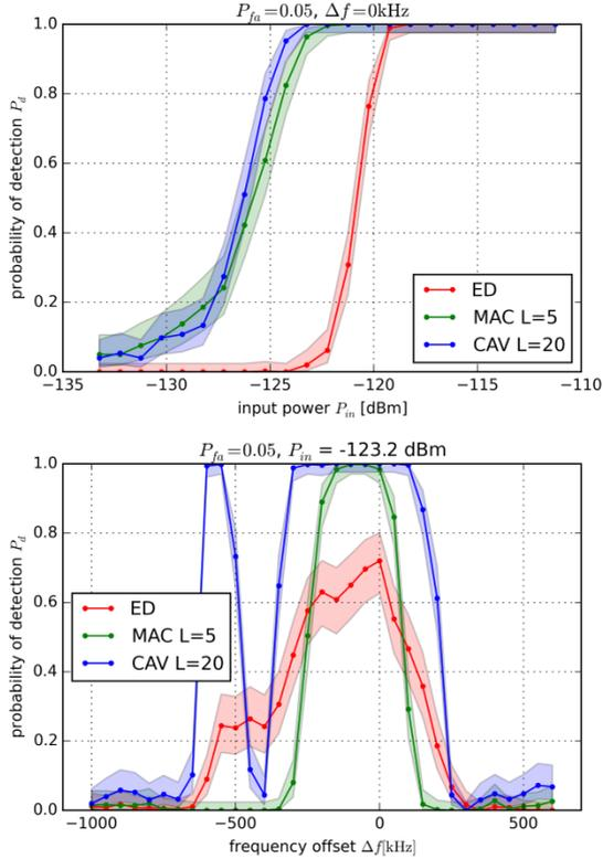
**Figure 3:** Probability of detection versus power (top) and frequency offset (bottom).
